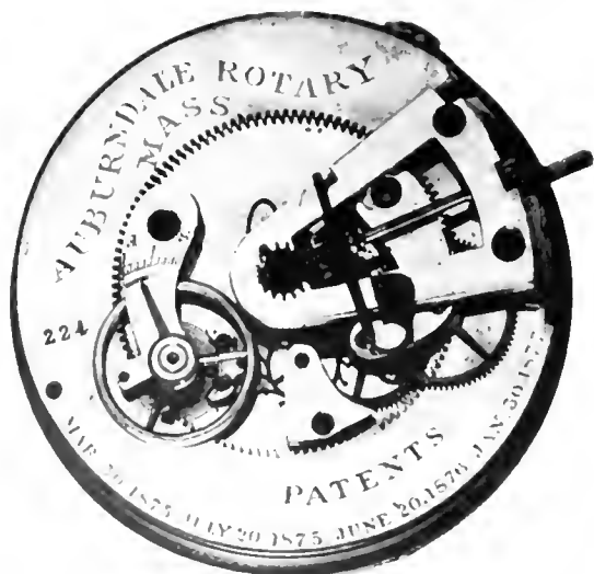
Figure 9. AUBURNDALE ROTARY WATCH MOVEMENT. (In the author's collection.)
